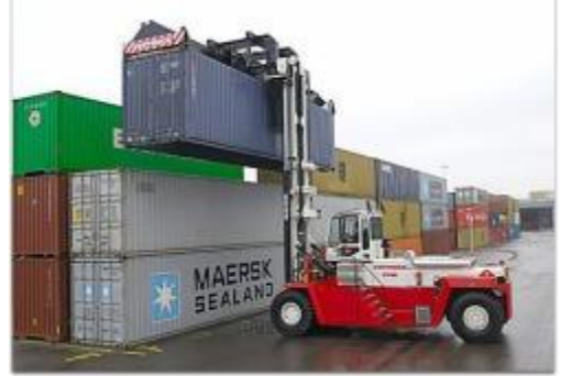
Xe nâng container hàng (loại chụp nóc) Loaded container handler (with top-lift spreader)
