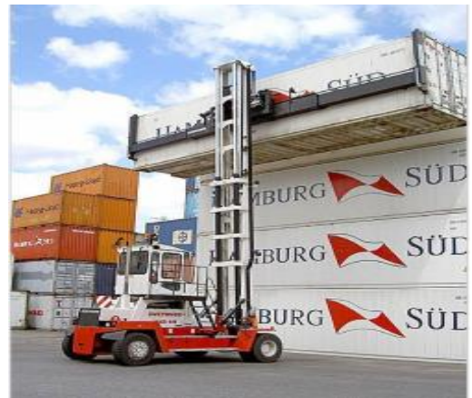
Xe nâng vỏ container (loại kẹp cạnh) Empty container reach-stacker (with side-lift spreader)
